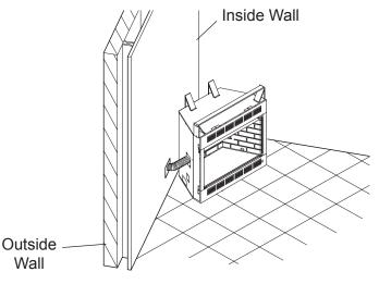
Figure 19 - 45° Corner Installation on Slab Floor
